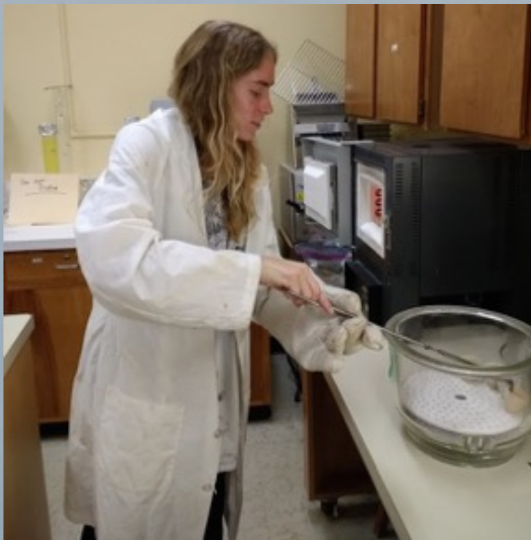
Figure 3: Soil sample prior to measurement. Figure 4: Samples being placed in 950°C oven.
