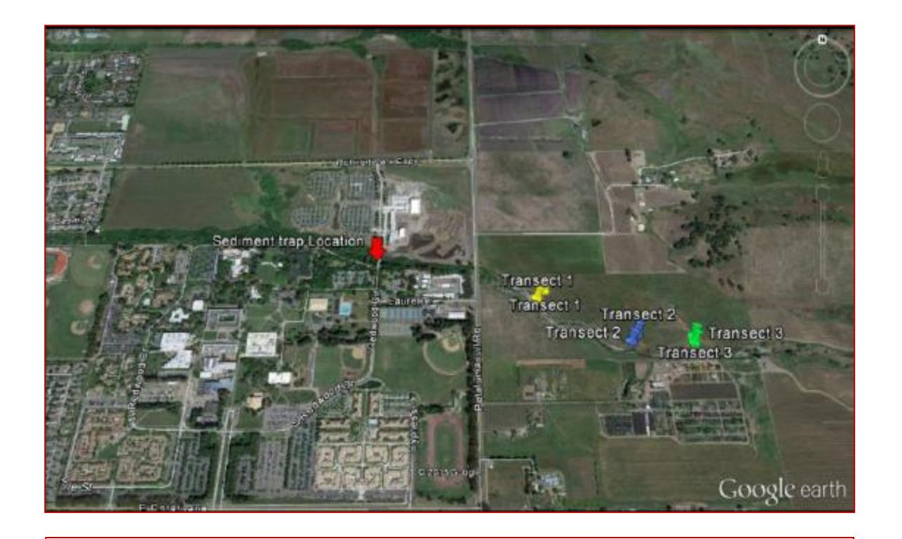
Site map: The three cross-sectional surveys are located on Copeland Creek's alluvial fan. The sediment traps will be installed in the channelized portion of the creek near the bridges leading to the Green Music Center.
