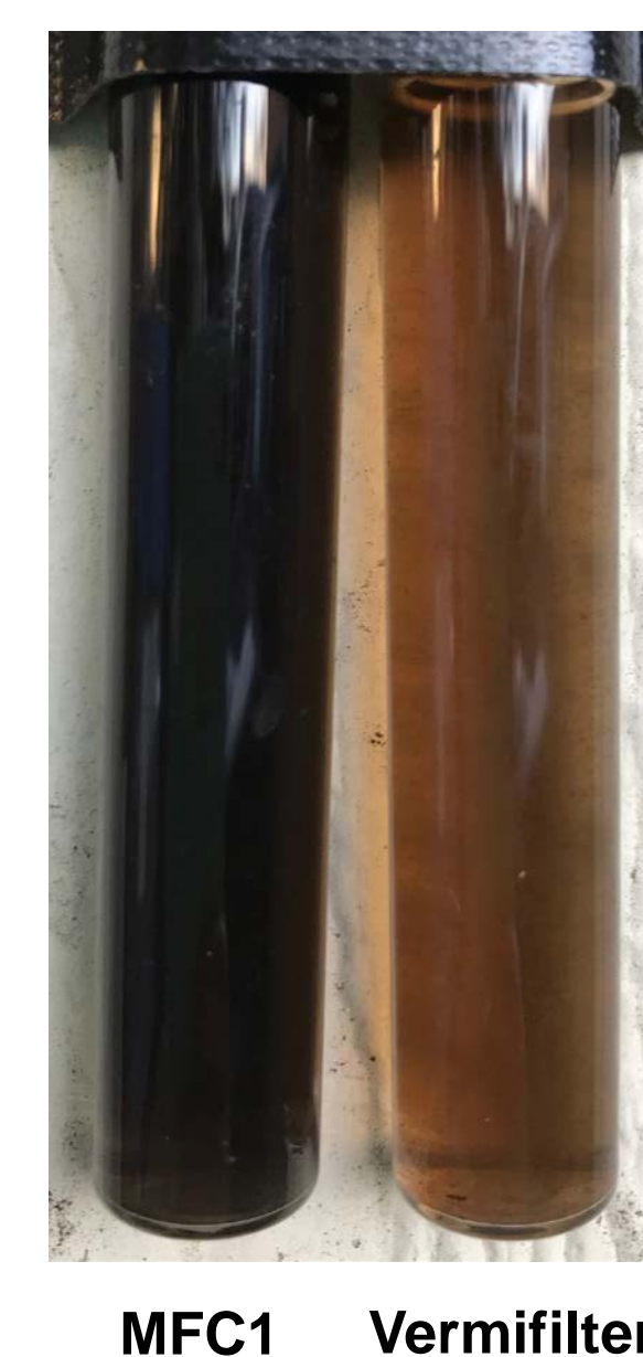
Fig. 2. Concentrations of phenolics in water flowing through the Vintners Square treatment system. Left: Tannins and polymeric anthocyanins; detection limit, 0.2 mg/L (Sample date, 5/14/2018). Right: Relative clarity of MFC1 effluent compared to effluent from the vermifilter.
