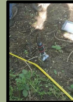
Figure 3: CO<sub>2</sub> Gas Probe in modified bottle. The modified bottle helps capture the released carbon dioxide gas.
