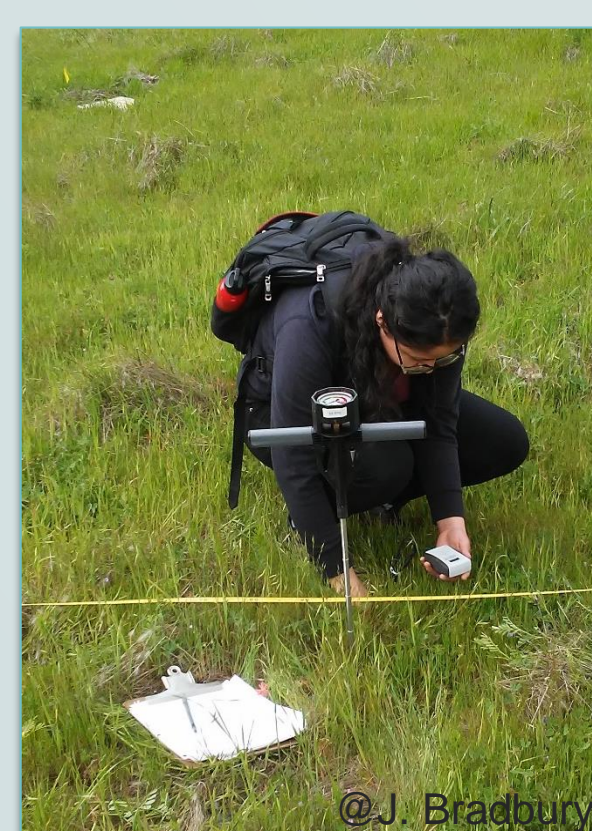
Measuring soil moisture and penetration resistance along transect
