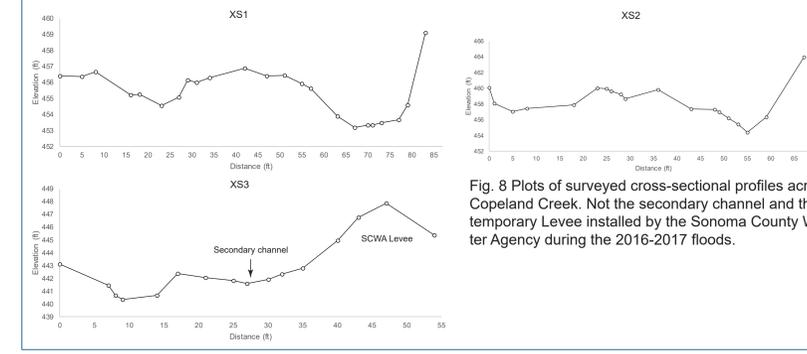
Fig. 8 Plots of surveyed cross-sectional profiles across Copeland Creek. Note the secondary channel and the temporary Levee installed by the Sonoma County Water Agency during the 2016-2017 floods.
