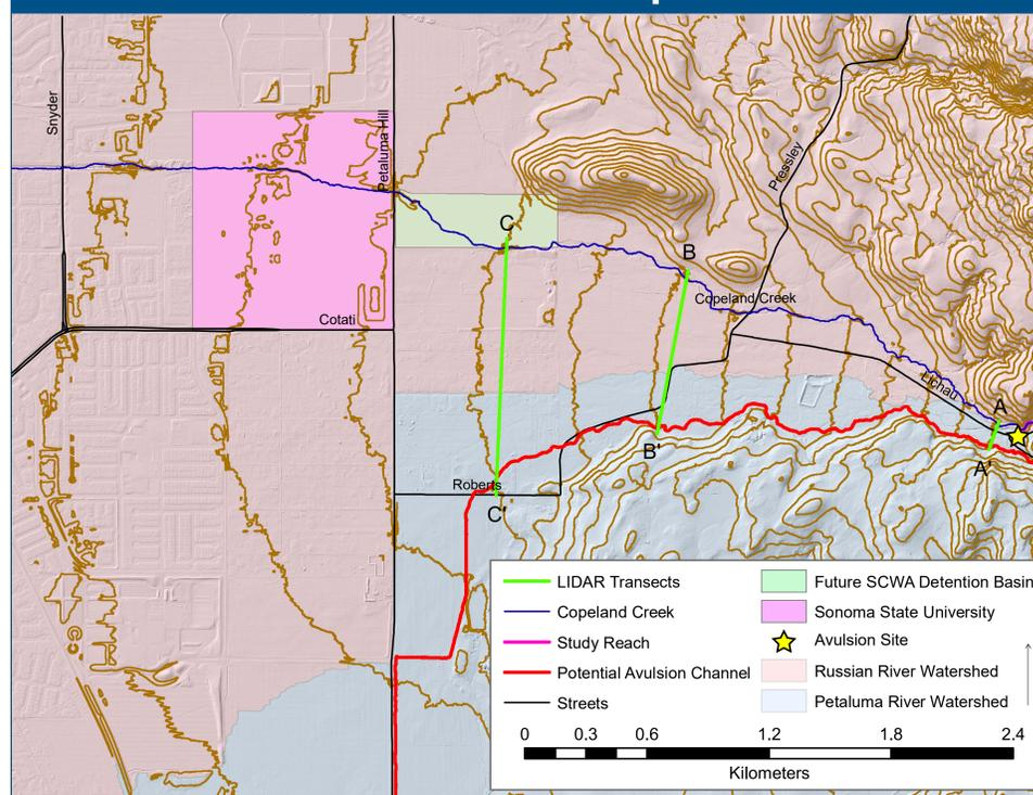
Fig. 2 Map of alluvial fan reach of Copeland Creek, displaying concentric topographic circles characteristic of alluvial fans. Potential avulsion channel, shown in red, drains into the Petaluma River watershed, where the current channel drains into the Laguna de Santa Rosa, part of the larger Russian River watershed. Study reach (pink) is area of figure 6.
