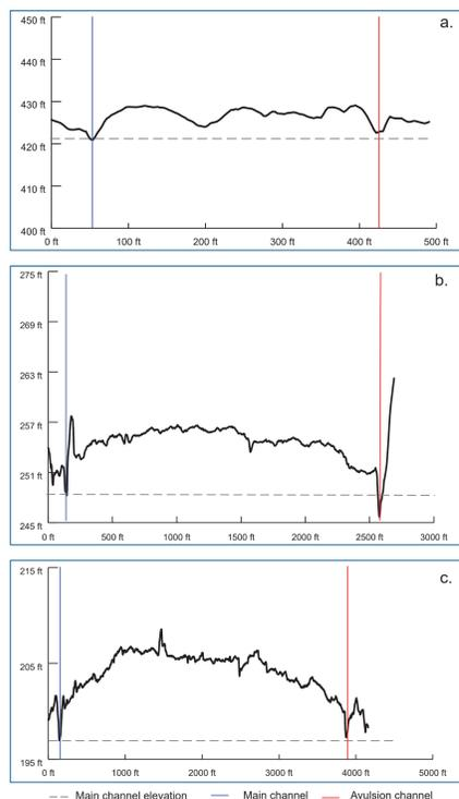
Fig. 3. Cross sectional profiles of Copeland Creek's alluvial fan derived from LIDAR data. a) A-A; vertical exaggeration ~ 5:1 b) B-B; vertical exaggeration ~64:1 c) C-C; vertical exaggeration ~12:1
