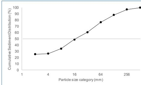
Fig. 4 Cumulative size distribution of bedding particles in Copeland Creek main channel, just below alluvial fan apex. D50 ~ 16 mm
