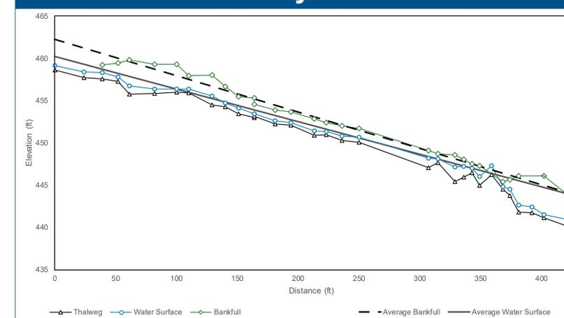
Fig. 7 Plot of surveyed longitudinal profile of Copeland Creek study reach. Note the average bankfull and average water surface lines converging in the downstream direction.
