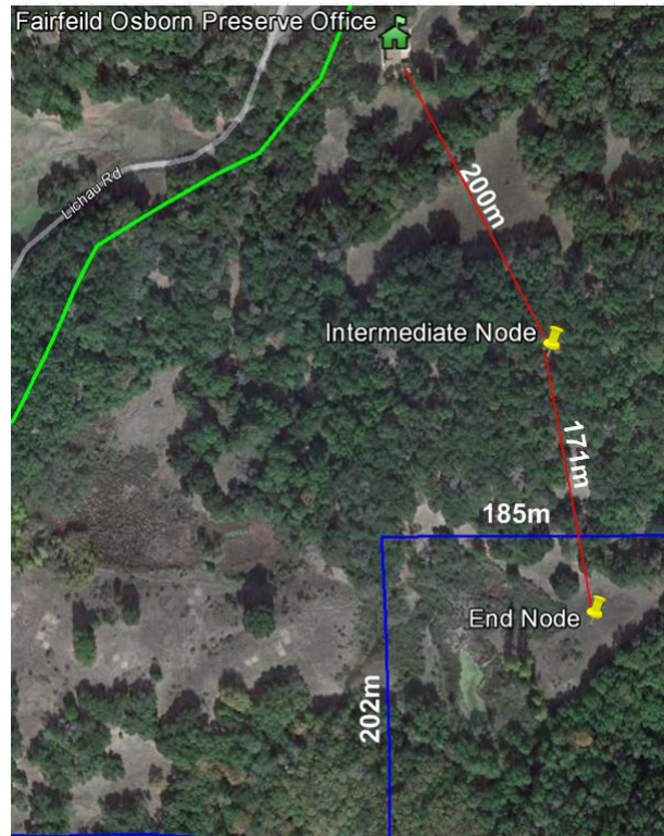
Figure 3 - Distances between Each Node & End Node Coverage
