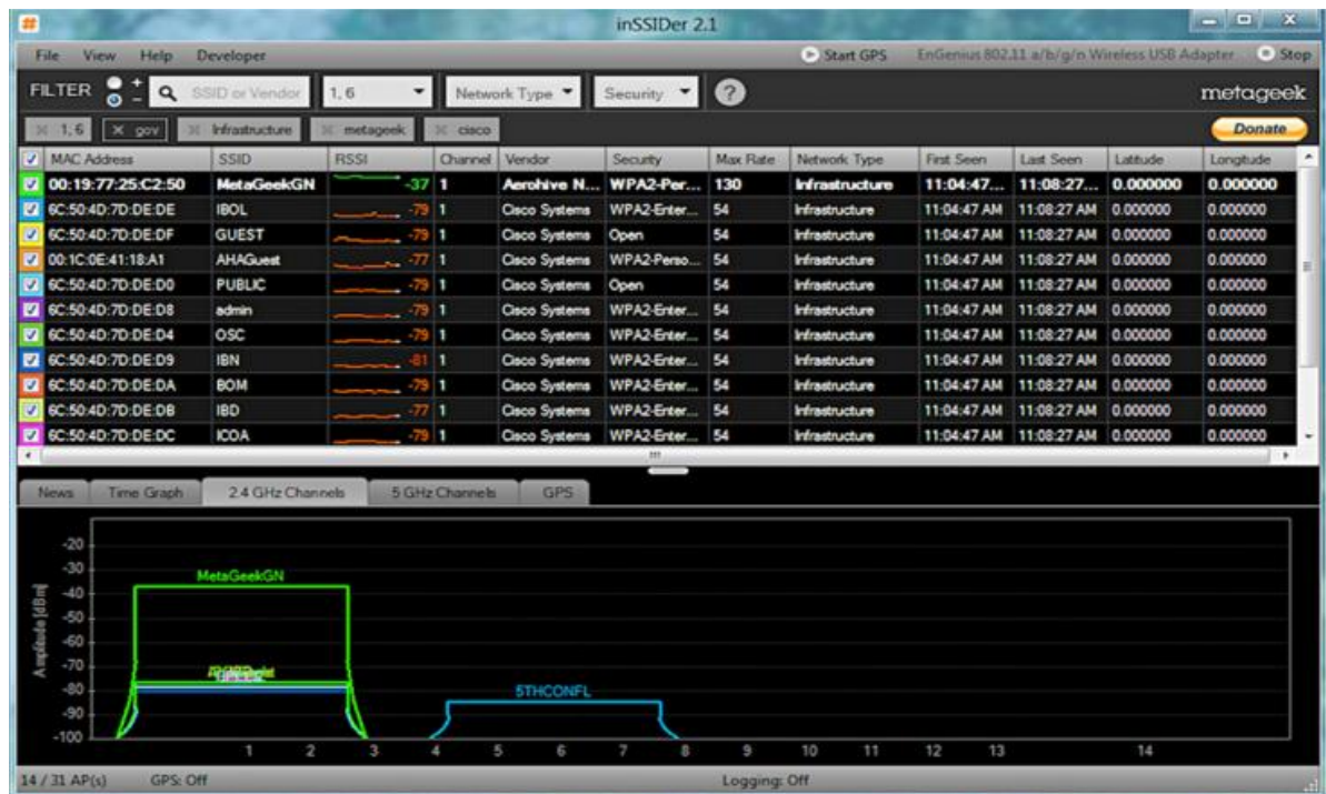
Figure 19 – The Wireless SSIDs Captured by InSSIDer [18]
